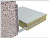
Now impale the insulation onto the spike as can be seen in this cross-section. Please note two spikes should be used for each piece, approx. 150mm inwards from each end.
