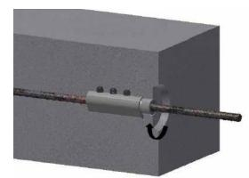
The male TSE should now be tightened using the calibrated torque wrench (see page 13).
