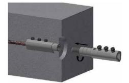
Once the concrete has cured sufficiently and the shuttering system has been removed the fixing plate is removed exposing the internally threaded section of the female coupler. The ALC-SKM (male) can be threaded in until the lock shear bolts come into a satisfactory alignment to allow access with the impact wrench.
