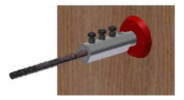
Attach the fixing plate to the shuttering system and screw the ALC-SKF (female) onto this. The rebar can now be inserted into this ensuring it reaches the stop pin. Once the bar is correctly inserted the lock shear bolts can be hand tightened.
