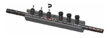
After confirming that the coupler is correctly aligned use the impact wrench (see page 13) to tighten the lock shear bolts, the bolts should be tightened on one side of the coupler first working from the central stop pin towards the outside edge of the coupler. When each bolt reaches the correct torque setting the head of the lock shear bolt will shear off. Complete this process for both sides of the coupler and all couplers at the joint.
