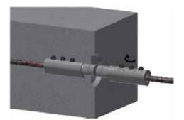
After confirming that the coupler is correctly aligned use the impact wrench (see page 13) to tighten the lock shear bolts, the bolts should be tightened in order working from the concrete face towards the outside edge of the coupler. When each bolt reaches the correct torque setting the head of the lock shear bolt will shear off. Complete this process for all couplers at the joint.
