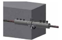
The locking rings should now be tightened using the calibrated torque wrench (see page 13) against both the female and male section of the coupler. The continuity steel can now be inserted into the coupler and the lock shear bolts can be tightened by hand.
