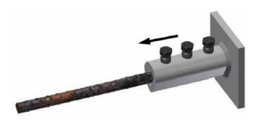
Slide the Headed Anchor Alligator Coupler over the end of the reinforcement steel that requires the anchorage until it comes to rest, ensuring the rebar has made full contact with the back plate. The lock shear bolts should be tightened by hand to stabilise the coupler.
