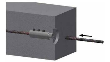
Once the concrete has cured sufficiently and the shuttering system has been removed the fixing plate is removed exposing the internally threaded section of the female coupler. The male TSE threaded coupler is threaded in until hand tight.
