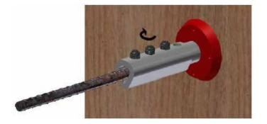
After confirming that the coupler is correctly aligned use the impact wrench (see page 13) to tighten the lock shear bolts, the bolts should be tightened in order working from the central stop pin towards the outside edge of the coupler. When each bolt reaches the correct torque setting the head of the lock shear bolt will shear off. The concrete can now be poured.
