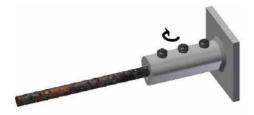
After confirming that the coupler is correctly aligned use the impact wrench (see page 13) to tighten the lock shear bolts, the bolts should be tightened working from the back plate working towards the outside edge of the coupler. When each bolt reaches the correct torque setting the head of the lock shear bolt will shear off. Complete this process for all couplers at the joint.
