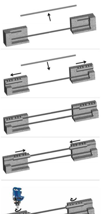
Firstly remove the rejected section of rebar, ensuring that a length of suitable concrete free reinforcement steel is left exposed at each side of the cut to accommodate at least the length of the corresponding Alligator Coupler of the equivalent bar diameter. The replacement length of reinforcement steel should be cut to a length 10mm less than the resultant gap in the reinforcement steel to allow easy installation.
