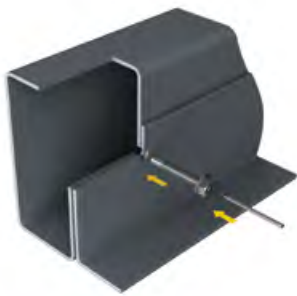
Bolt assembly placed in hole
