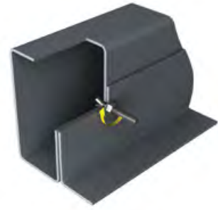
Tighten bolt to recommended torque
