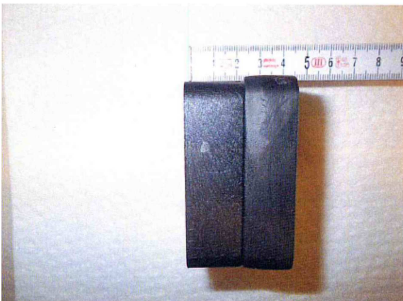
Fig. 2: Mounting plate UP 20 NA lightweight after maximum stress, with distinctly discernible deformation in the plate on the right.
