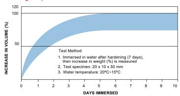
Tests were carried out on a sample of Leakmaster measuring 20 x 10 x 50 mm. The sample was left to harden for seven days before immersion in water at a temperature between 15 and 20 degrees Centigrade.
