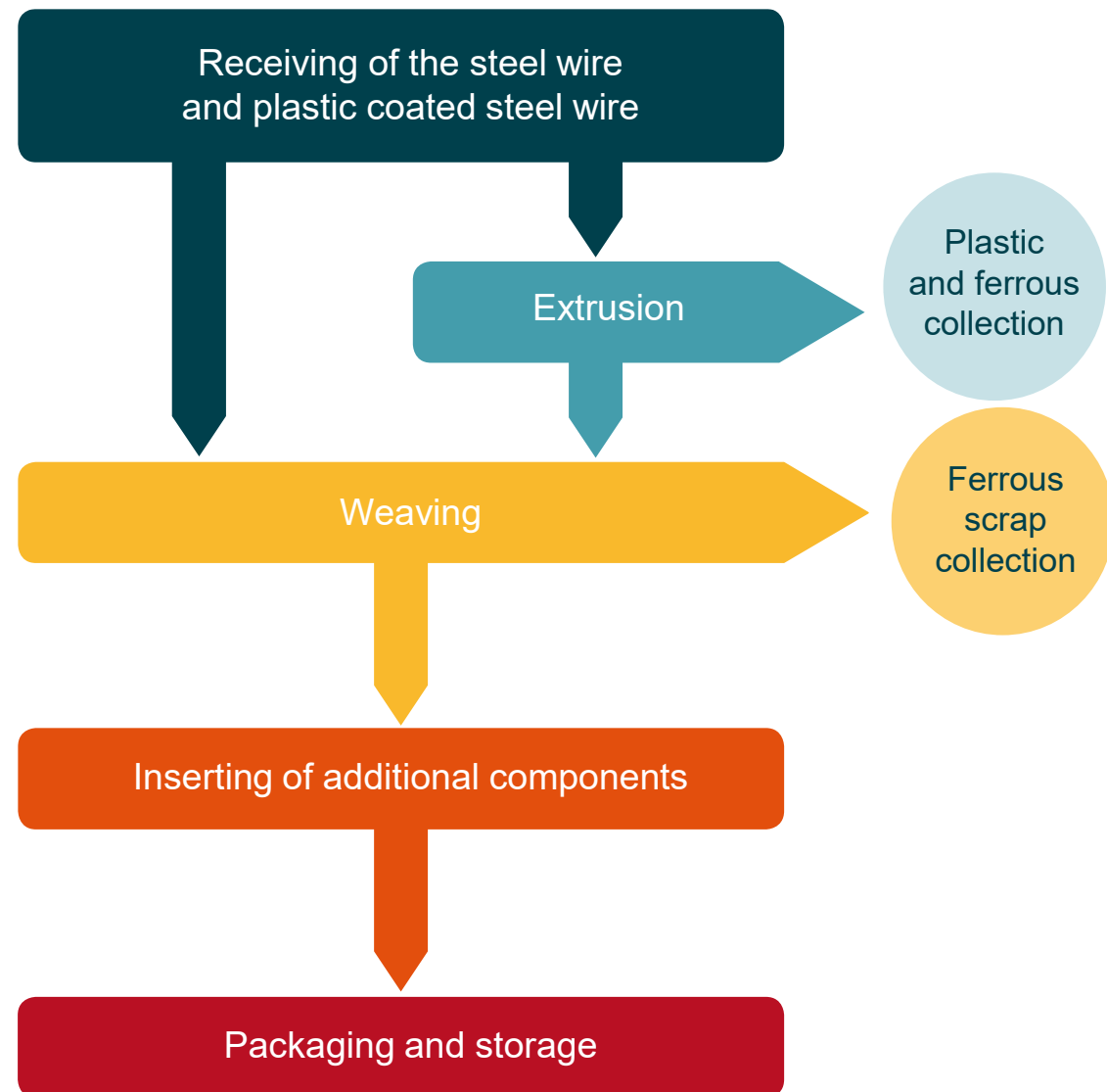
Figure 4: Production process of the Gabions
