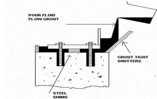
Grout should be chamfered to ensure that unrestrained shrinkage cracking does not occur.
