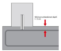
No additional lap joint protection is required when subjected to pressures of up to 3 m hydrostatic head. If exposed to pressurised water > 3 m and  $\leq$  20 m hydrostatic head, the lap joints between the **contecSEAL 150** metal waterstops must be additionally secured with the supplied contaflexactiv VAS 50/150 sealing strips.
