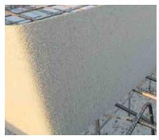
composite system for fresh concrete with a very strong bond to concrete. The surface-enlarging coating results in an extreme increase in the leak path, furthermore the effect of fresh concrete sintering into the adhesive composite layer is initiated.
